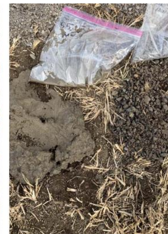
MW-3 transition to greenish brown thick silty clay
