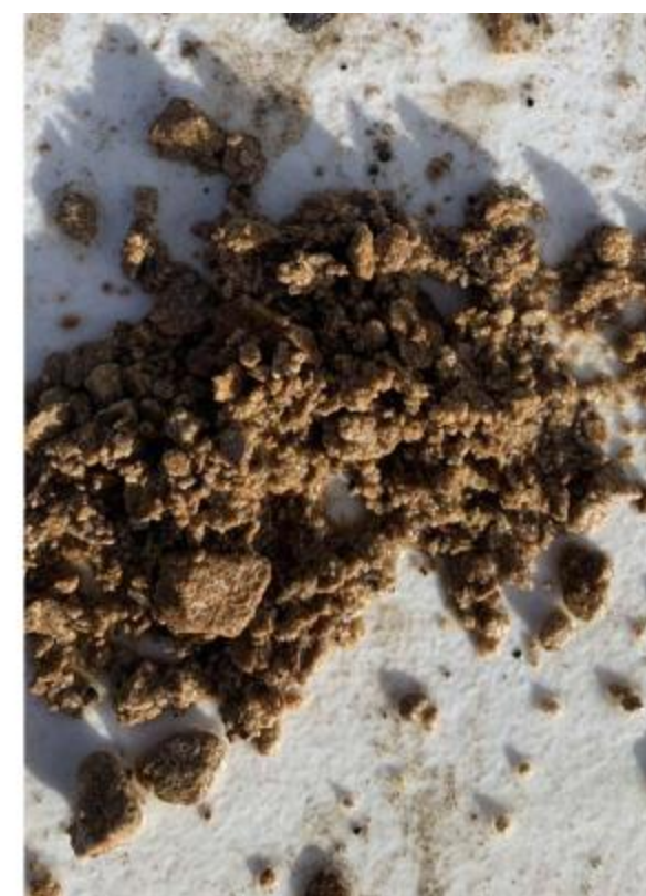
Sandstone and shale cuttings from MW-1
