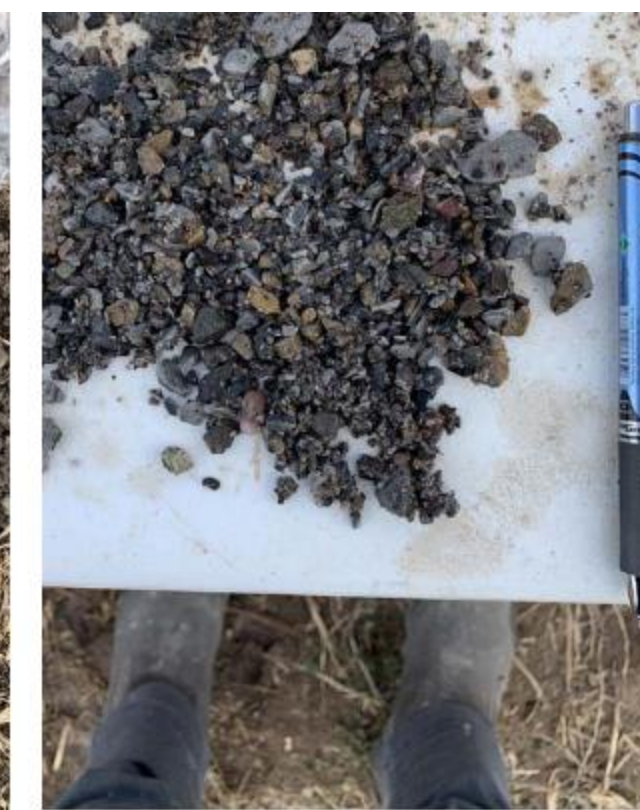
MW-3 shale and sandstone cuttings
