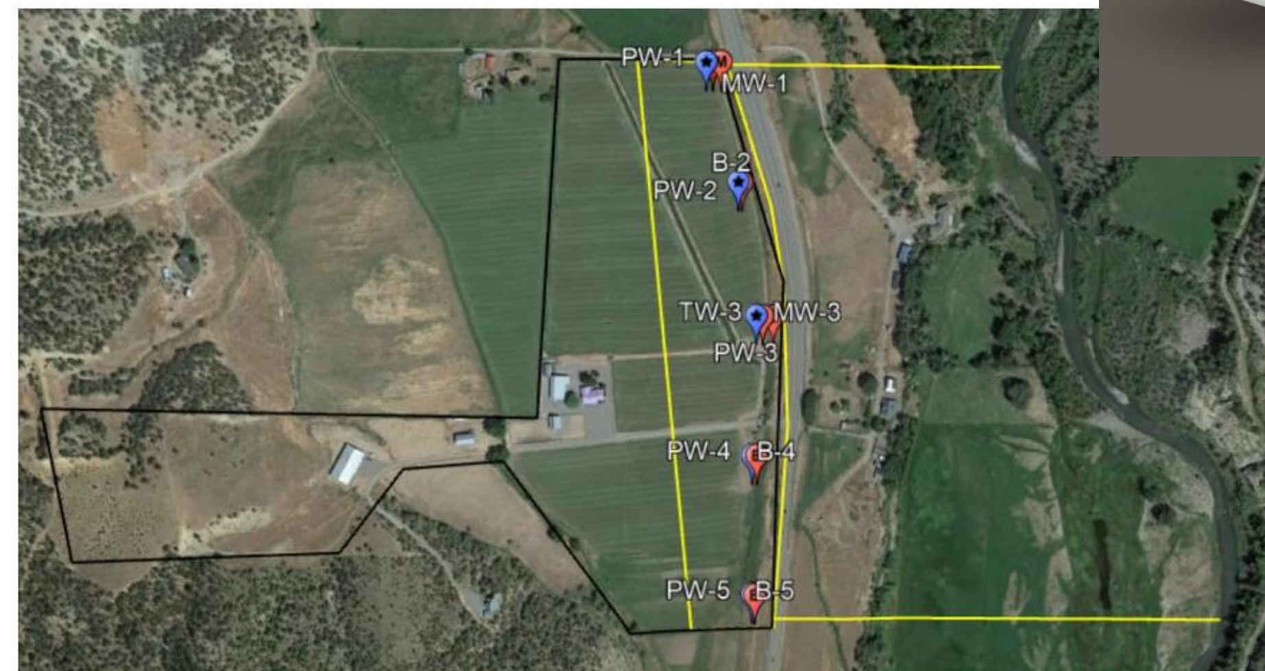
Figure 1 – RBF project site property boundary map (black polygon) with primary geophysics surveying areas of interest indicated with the yellow polygon and two river profiles extending east towards the Uncompahgre River. The conceptual well layout is also included in the figure, with tentative well placements indicated with red and blue pins.
