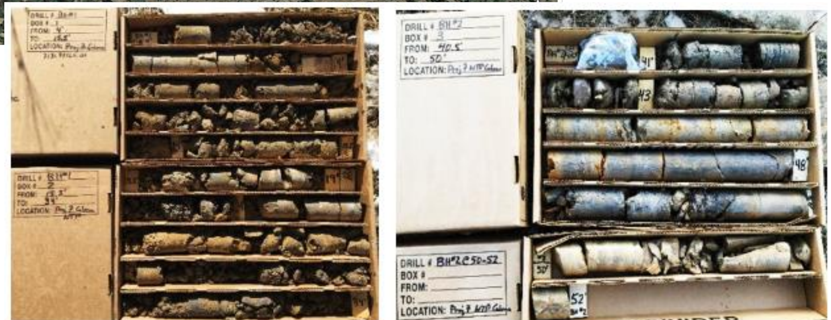
Figure 3 (left) are the rock core samples from BH#1 at 4 to 34 feet. Figure 4 (right) are the core samples from BH#2 at 40.5 to 52 feet.
